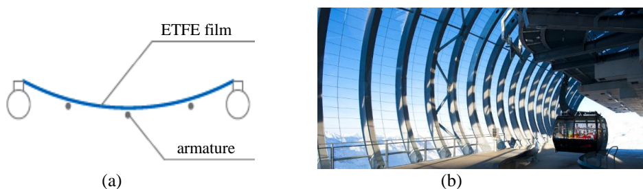
Fig. 5 a) Cross section of single layer ETFE film panel; b) Gaislachkogel gondola [17];
