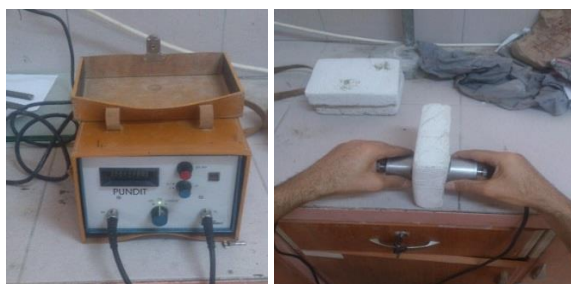
Fig. 3. The experimental setup for measuring ultrasonic pulse velocity
