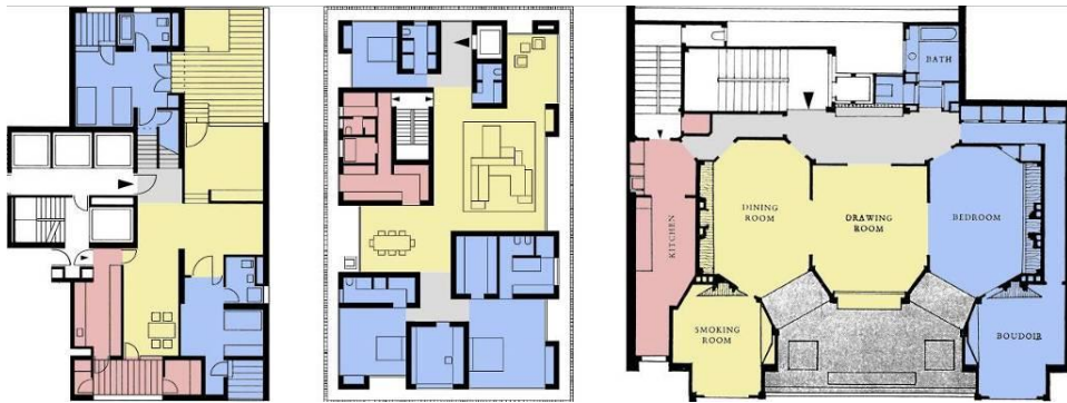
Fig. 4 Characteristic apartments with auxiliary entrance through the kitchen: 1) Kanchanjunga tower, Mumbai (Charles Correa Associates, 1983), 2) Ninetree Village, Hangzhou (David Chipperfield Architects, 2008), 3) Rue Franklin Apartments, Paris (Auguste Perret, 1904) (Source: author's archive)
