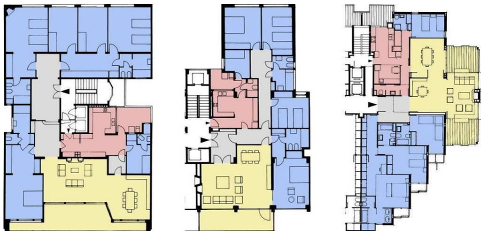
Fig. 5 Characteristic apartments with auxiliary servants' entrance: 1) Apartment building at Carrer del Mestre Nicolau, Barcelona (Francesc Mitjans, 1960), 2) Seida building, Barcelona (Francesc Mitjans, 1962), 3) Banco Urquijo, Barcelona (José Antonio Coderch, 1967) (Source: author's archive)
