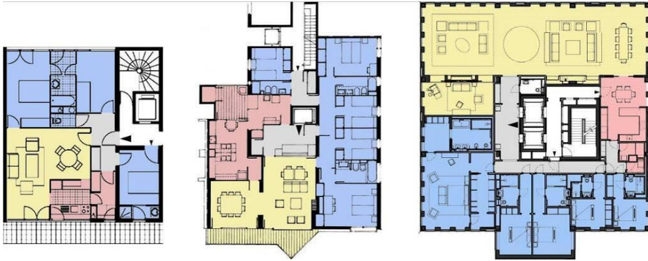
Fig. 6 Characteristic apartments with auxiliary entrance through individual space: 1) Cité Descartes, Marne-la-Vallée (Yves Lion, 1995); 2) Housing in J. S. Bach street, Barcelona (José Antonio Coderch, 1957); 3) Holland Green, London (OMA & Allies & Morrison, 2016) (Source: author's archive)
