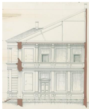
Fig. 6 The cross-sectional design of the hotel “Hungaria” ballroom, built in 1882 (HAS, F:2, ép. eng. IV kör 10/1882.)
