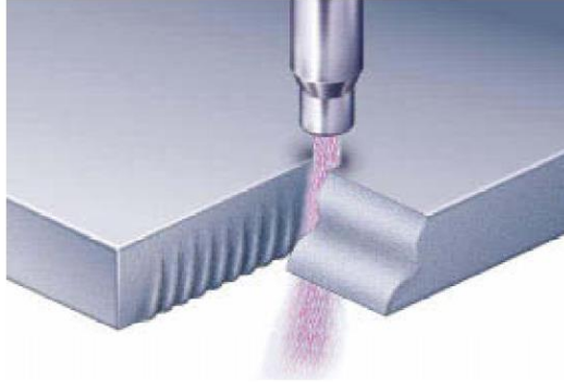
Fig. 2 Development of the cut surface by abrasive water jet cutting
