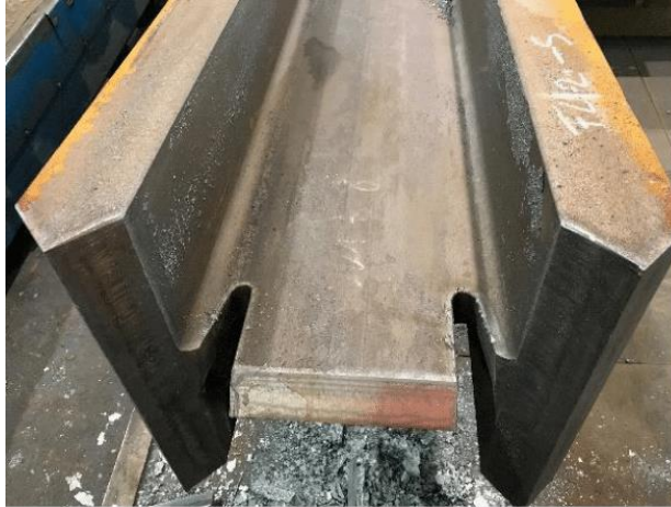
Fig. 6 Beam with weld access holes
