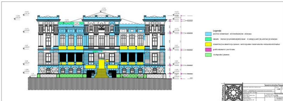
Fig. 4 "Karađorđev dom", main façade (northeast) deterioration mapping, author: E.V.Petrović (November 2020)
