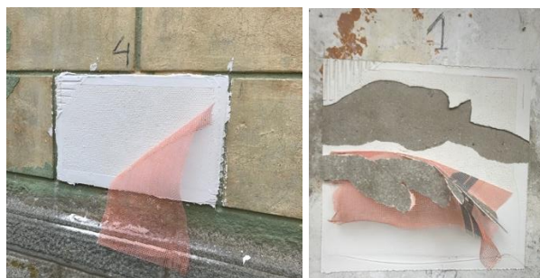
Fig. 6 “Karadorđev dom”, “pull-off” test results (test No4)-left, test results (test No1)-right, author: E.V.Petrović (November 2020)
