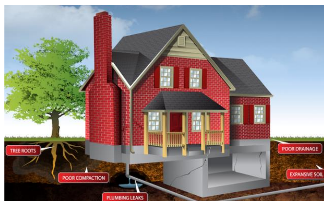
Fig. 2 Causes of damage of foundations and superstructure [1]
