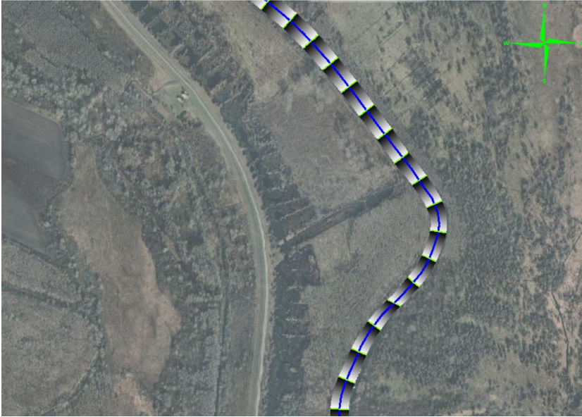
Fig. 7 Cross-sections in a part of the river reach used for creation of raster bathymetry DEM (RAS Mapper)
