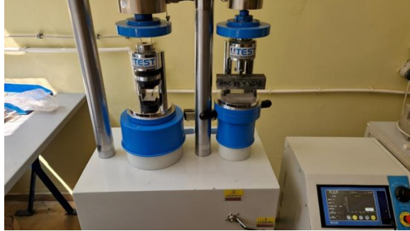
Fig. 2 Test setup for flexural strength testing
