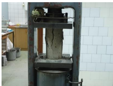
Fig. 3 Testing and results: a) Testing of compressive strength for the first series, b) Diagram of compressive strength for each series
