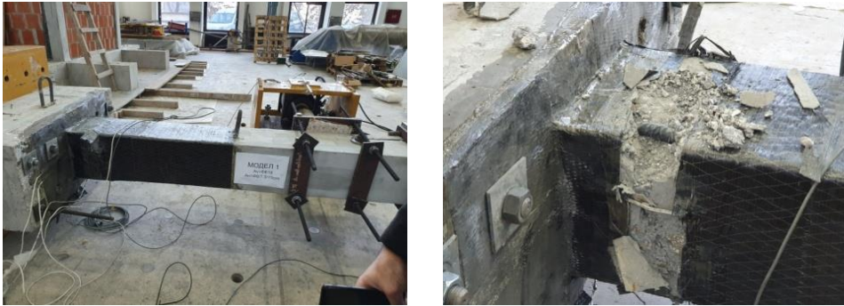
Fig. 5 Quasi-static tests of Model M1: a) Shot during the quasi-static testing of column Model M1; b) Damage from quasi static testing of column Model M1
