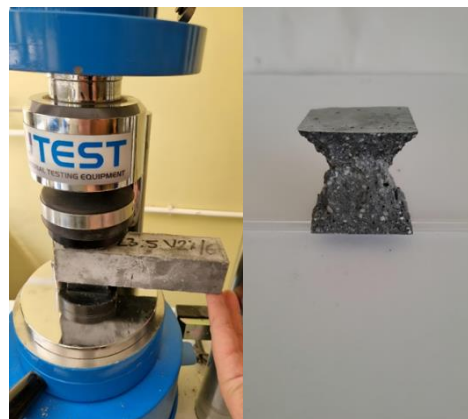
Fig. 4 Disposition during testing the compressive strength (left) and the appearance of the sample exposed to compression until failure (right)
