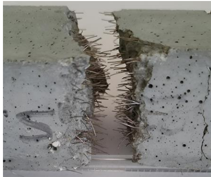
Fig. 3 Appearance of the concrete with steel microfibers at the failure point after testing the flexural strength
