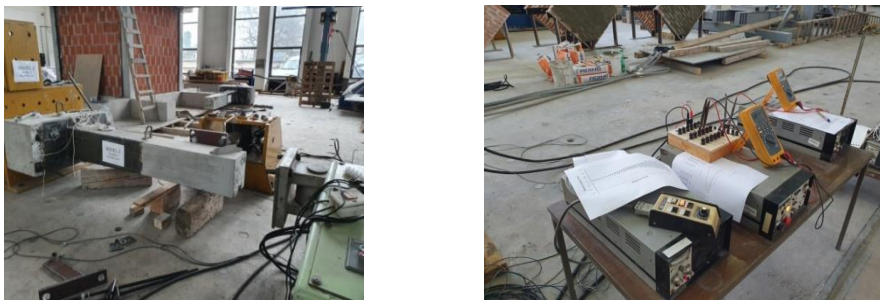
Fig. 6 Experimental set-up quasi static testing of column Model M2
