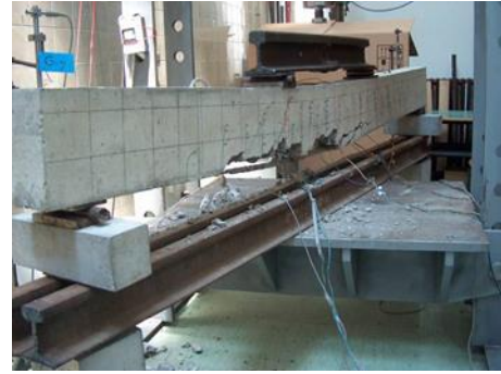
Fig. 7 Failure caused by loss of adhesion of CFRP reinforcement
