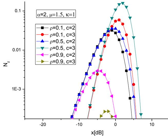
**Fig. 1** Normalized average level crossing rate versus normalized macrodiversity SC receiver output signal envelope for several values of parameter  $c$  and  $\rho$
