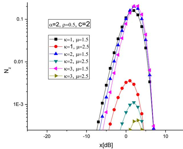
**Fig. 2** Normalized average level crossing rate in terms of normalized macrodiversity SC receiver output signal envelope for several values of Rician factor  $\kappa$  and parameter  $\mu$
