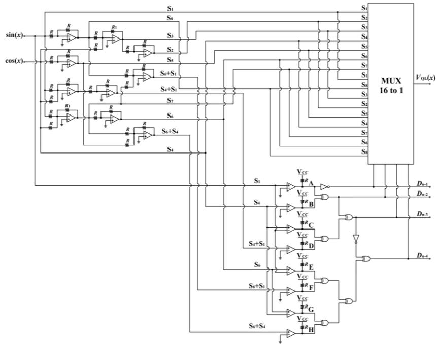
Fig. 1 A 4-bit mixed analog-digital circuit
