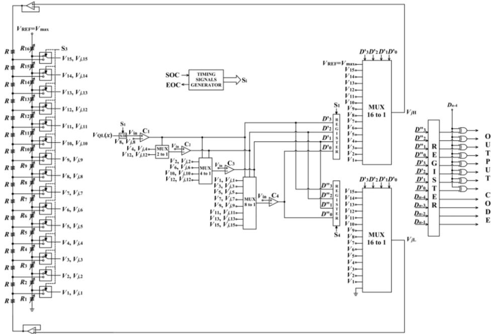
Fig. 3 An 8-bit two-stage nonlinear ADC of a compact design
