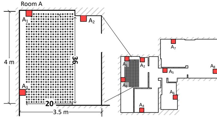
**Fig. 1** The map of the experimental environment with the red boxes denote anchor nodes
