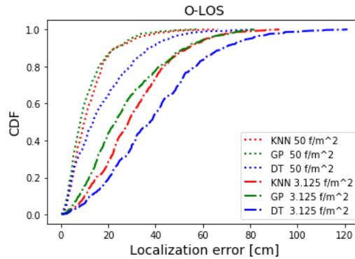
**Fig. 5** CDF of the localization errors of ML algorithms for 0-LOS case and fingerprint densities of  $50 f/m^2$  and  $3.125 f/m^2$
