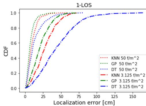
**Fig. 4** CDF of the localization errors of ML algorithms for 1-LOS case and fingerprint densities of  $50 f / m^2$  and  $3.125 f / m^2$
