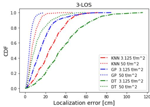
**Fig. 2** CDF of the localization errors of ML algorithms for 3-LOS case and fingerprint densities of  $50 f/m^2$  and  $3.125 f/m^2$
