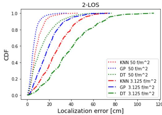
**Fig. 3** CDF of the localization errors of ML algorithms for 2-LOS case and fingerprint densities of  $50 f / m^2$  and  $3.125 f / m^2$
