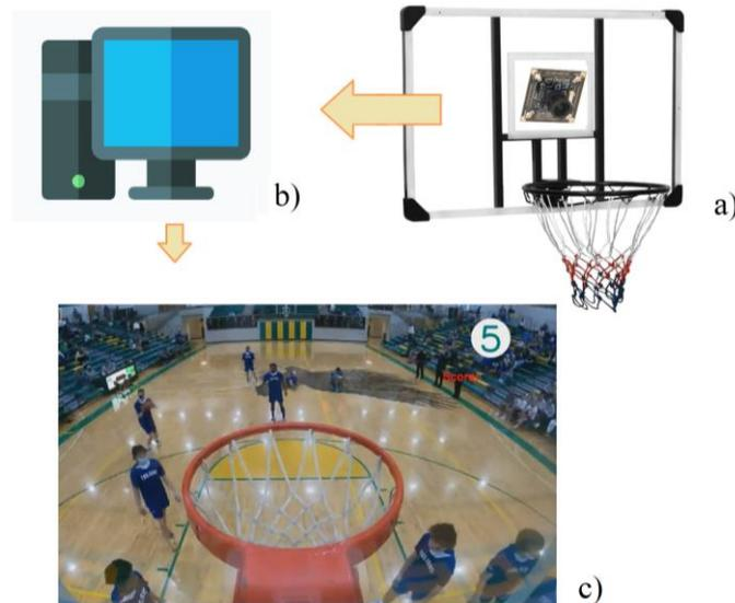
**Fig. 1** Functional scheme of Vision Based Basketball Score Tracking System: a) Image acquisition using 2MP camera module with the wide-angle lens; b) Data processing; c) Output results presented within the camera view
