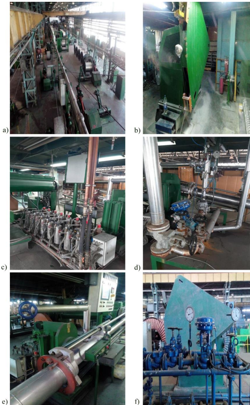
Fig. 3 a) Rope unwinding, part of the tube for vulcanization and winding, b) main traction (capstan) device, c) extruder with tempering system, d) steam injection, e) tube closing system, f) water inlet and traction (capstan) device at the exit from the tube
