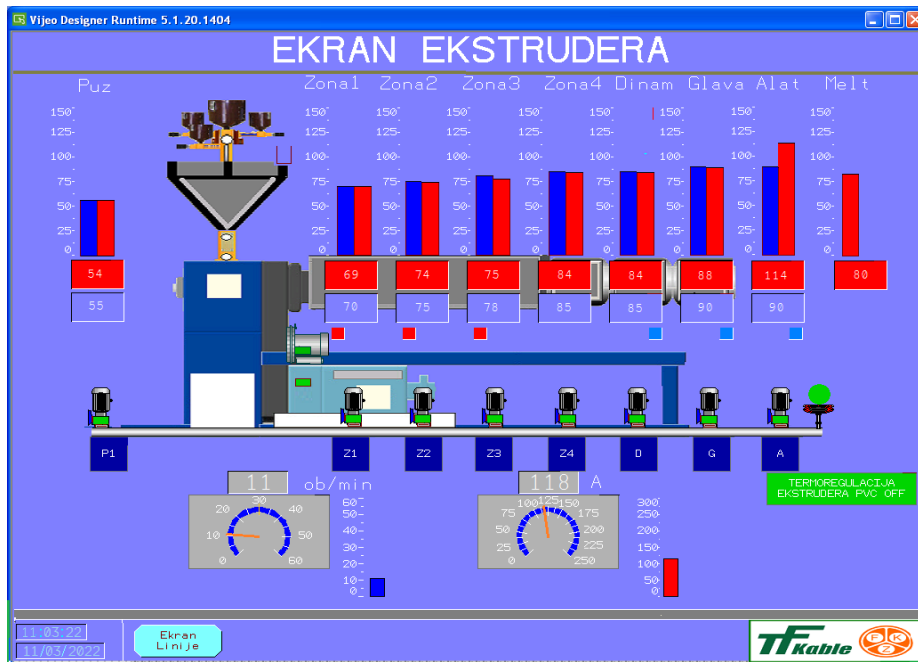
Fig. 9 Technological diagram of all parts of the system for driving and tempering the extruder (HMI screen)
