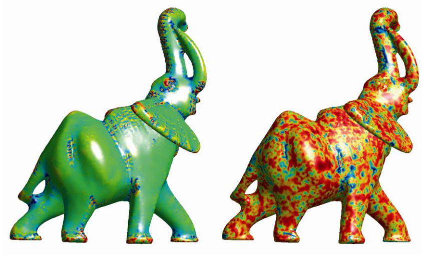
Fig. 4 The plot of Gaussian and mean curvature estimation computed by local differential geometry method.
