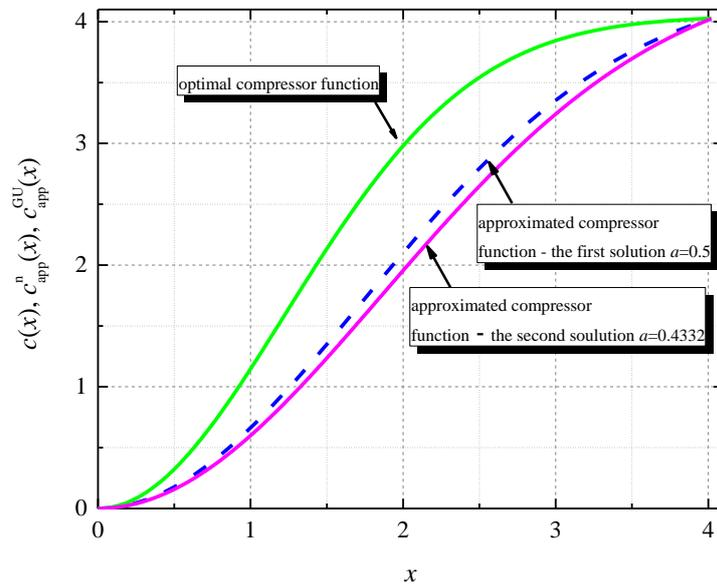
**Fig. 3** Optimal compressor function  $c(x)$ , the novel approximated compressor function  $c_{\text{app}}^n(x)$ , the approximated compressor function with GU approximation  $c_{\text{app}}^{\text{GU}}(x)$ , for Gaussian PDF of unit variance,  $N = 128$ ,  $x_{\text{max}} = 4.0274$
