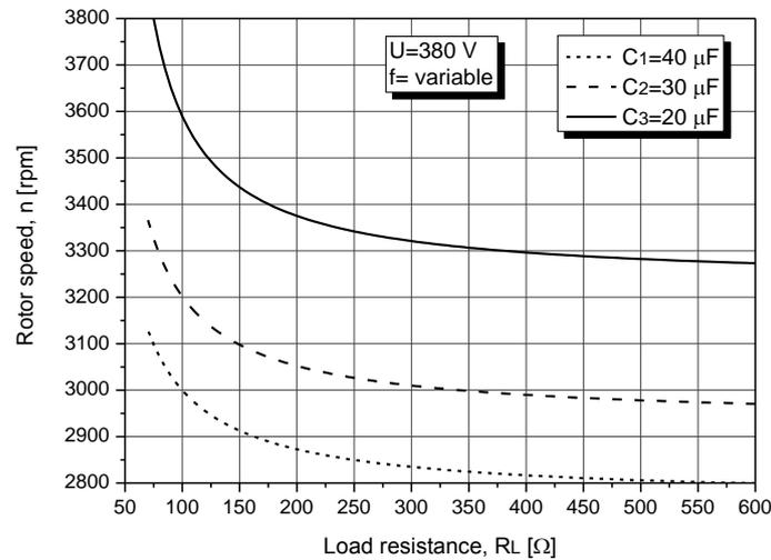
**Fig. 4** Computed regulation curves  $n = f(R_L)$ , while  $C = const$ , for constant voltage and variable frequency operation
