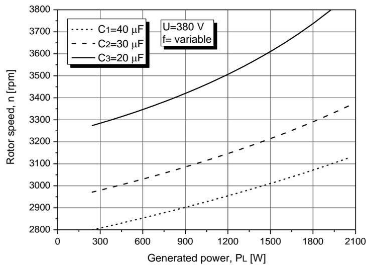
**Fig. 5** Computed regulation curves  $n = f(P_L)$ , while  $C = const$ , for constant voltage and variable frequency operation
