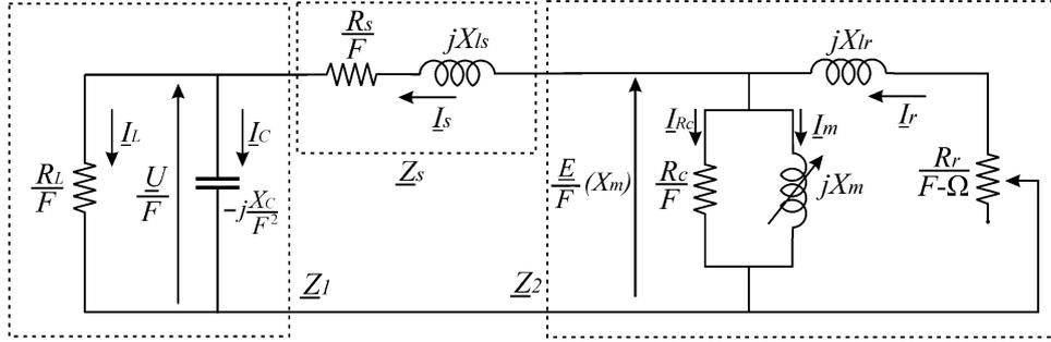
**Fig. 1** Modified equivalent circuit of induction machine, suitable for analysis
