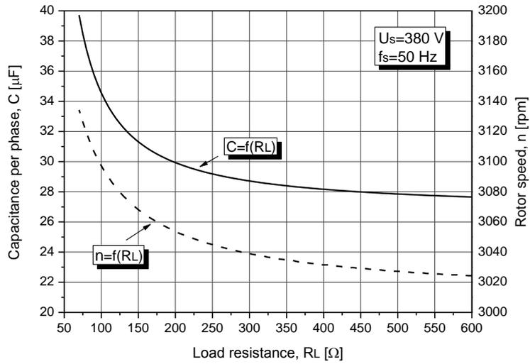
**Fig. 2** Regulation curves for constant voltage and constant frequency operation
