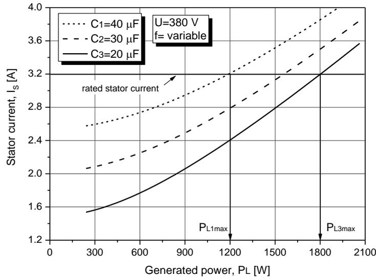
**Fig. 6** Computed stator current for constant voltage regulated by speed of a turbine and variable frequency operation
