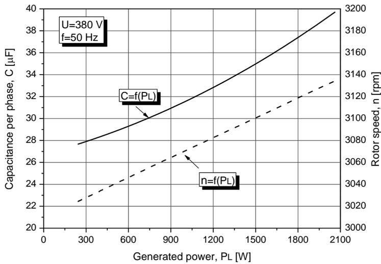
**Fig. 3** Constant voltage and constant frequency operation regarding generated power
