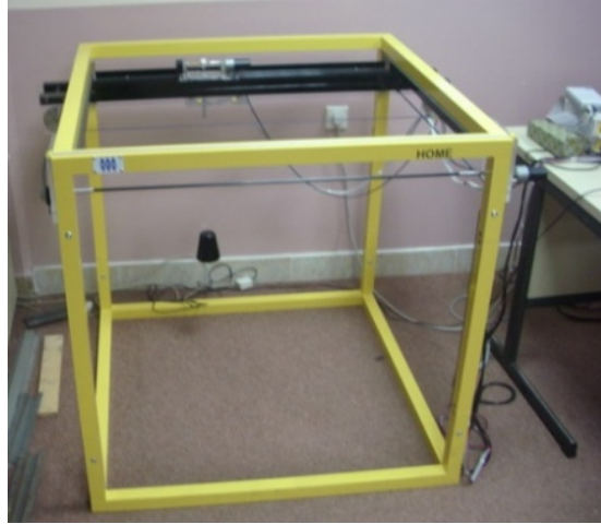
Fig. 1 The 3D crane system manufactured by Inteco
