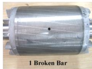
Fig. 4 A rotor with one fully broken bar.
