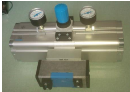
Fig. 8 Pneumatic booster Festo DP 63-10
