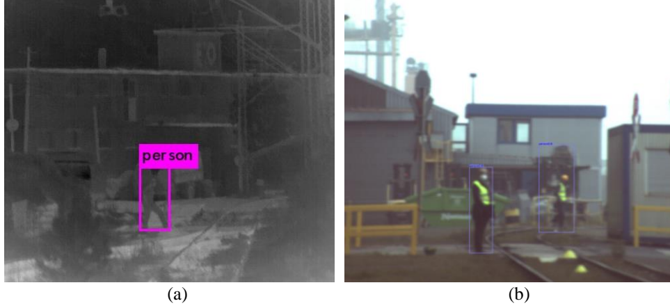
Fig. 2 DL-based object detection in railway scenes captured by thermal (a) and RGB camera (b).
