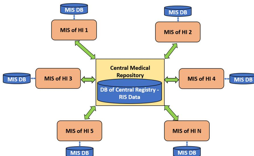
**Fig. 1** Radiological Information System (RIS) data are located only in the central registry database
