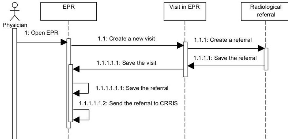
Fig. 12 The sequential diagram – the creation of radiology referral
