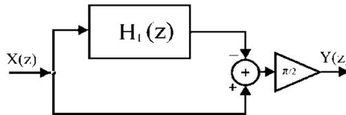
**Fig. 1** Differentiator configuration realized applying first order all-pass filter. Input and output signals are represented with their z transforms
