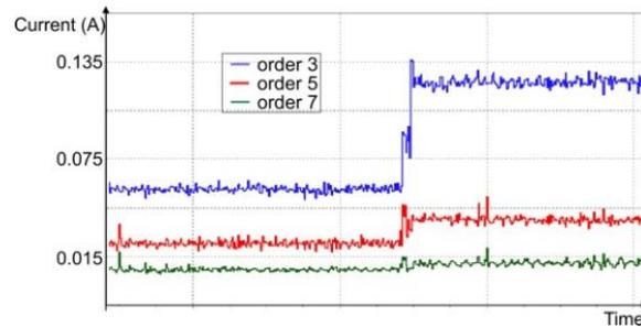
**Fig. 1** Current harmonic waveforms related to switching on a fluorescent lamp
