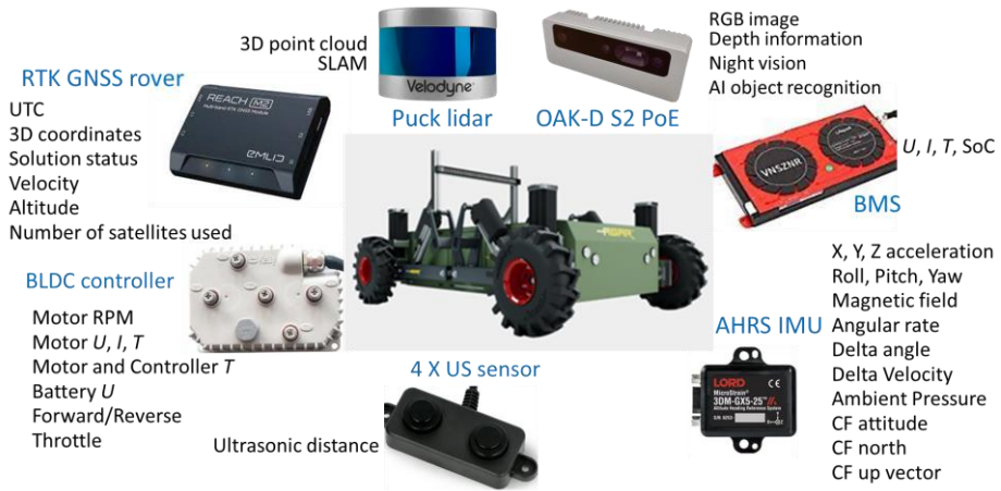
Fig. 3 AgAR sensor set and data gathered by a digital twin
