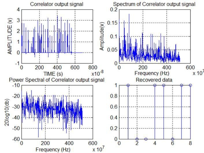
**Fig. 11** The correlator output signal with its power spectral, the spectrum and the data recovered
