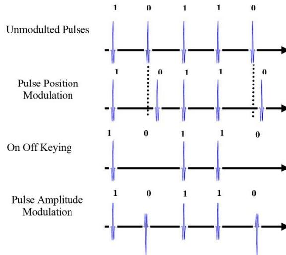
**Fig. 3** Modulations associated with UWB systems
