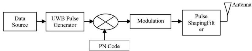
**Fig. 2** Block diagram of a DS-UWB signal generator
