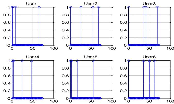
Fig. 4 Positions of chips at "1" of the code POC (73,4)
