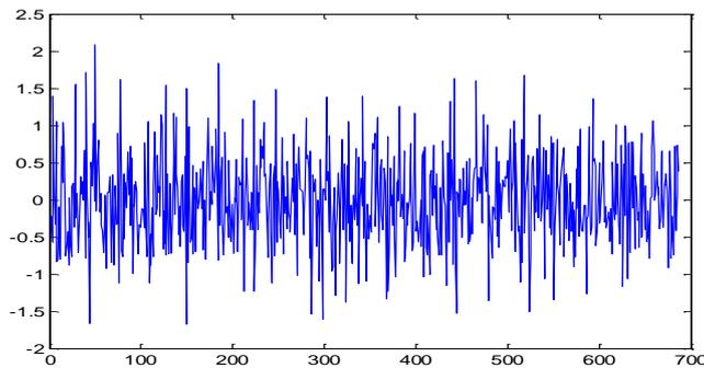
Fig. 9 AWGN Channel output, where  $E_b/N_0=2\text{dB}$
