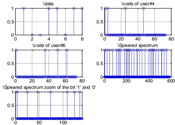
Fig. 6 Spread spectrum phase for the data sequence "10011011"
