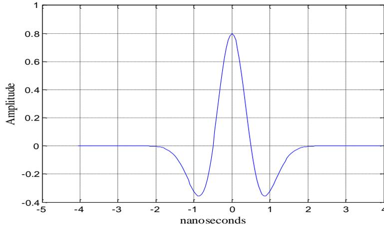
**Fig. 1** Second derivative of a Gaussian pulse
