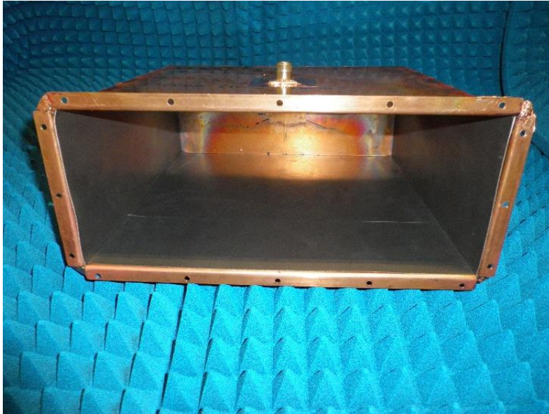
Fig. 6 Photography of the physical model of D metal enclosure with the EMI absorbers on lower wall and both side walls of enclosure (LW+2SW)
