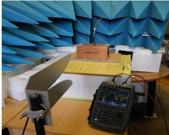
Fig. 4 Photography of measuring configuration used in a semi-anechoic room: transmitting antenna, VNA and EUT (enclosure D with a receiving antenna)
