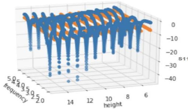
Fig. 10 Multiple Regression Predictions versus Actual  $S_{11}$
