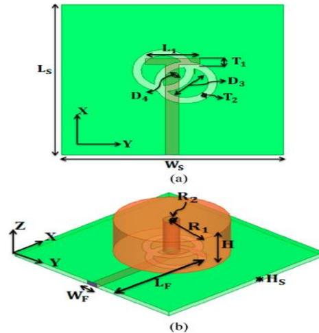
**Fig. 1** Structural Layout of DRA Antenna: a) Dual linked circular ring aperture; b) Panoramic view
