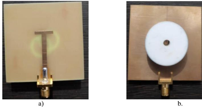
**Fig. 2** Fabricated prototype of proposed CP Antenna: (a) Bottom View; (b) Top View
