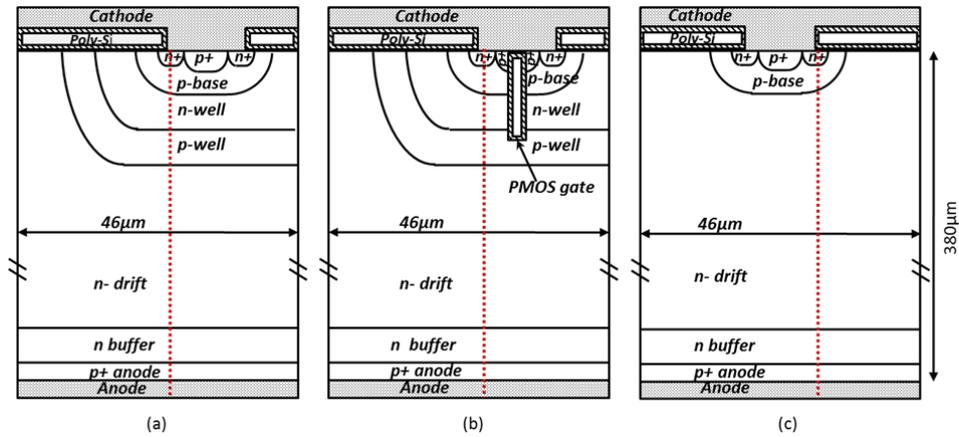
**Fig. 1** Schematic Structure diagram of (a) planar gate CIGBT, (b) planar gate CIGBT with deep PMOS trench channel and (c) conventional planar gate IGBT.
