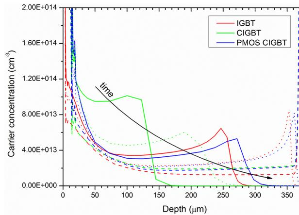
**Fig. 6** Simulated effective carrier concentration of structures based on the results shown in Fig. 5 (solid line: time=200ns, dotted line: time=400ns, and dash line: time at maximum anode voltage).
