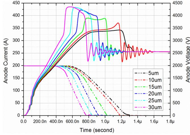
**Fig. 7** CIGBT turn-off waveforms with variable N-buffer thickness from  $5\mu\text{m}$  to  $30\mu\text{m}$  ( $V_{DC}=2500\text{V}$ ,  $I_a=200\text{A}$ ,  $T_j=25^\circ\text{C}$ ,  $R_g=0\Omega$ ).
