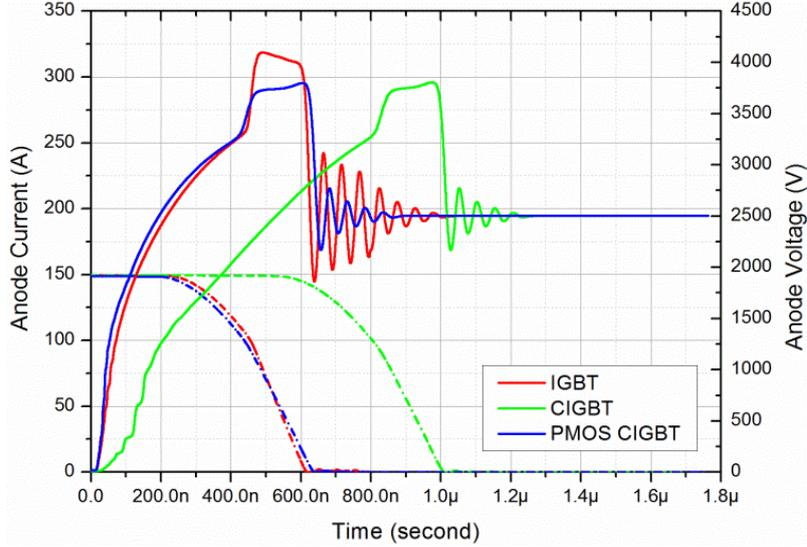
**Fig. 3** IGBT and CIGBT turn-off waveforms ( $V_{DC}=2500V$ ,  $I_a=150A$ ,  $T_j=25^\circ C$ , solid line: anode voltage; dashed line: anode current).
