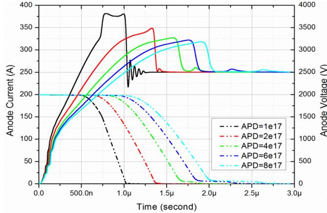
**Fig. 8** CIGBT turn-off waveforms with variable anode peak concentration ( $V_{DC}=2500\text{V}$ ,  $I_a=200\text{A}$ ,  $T_j=25^\circ\text{C}$ ,  $R_g=0\Omega$ ).
