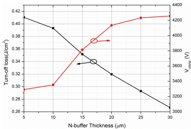
**Fig. 10** Turn-off loss and clamped voltage dependence on the N-buffer thickness.
