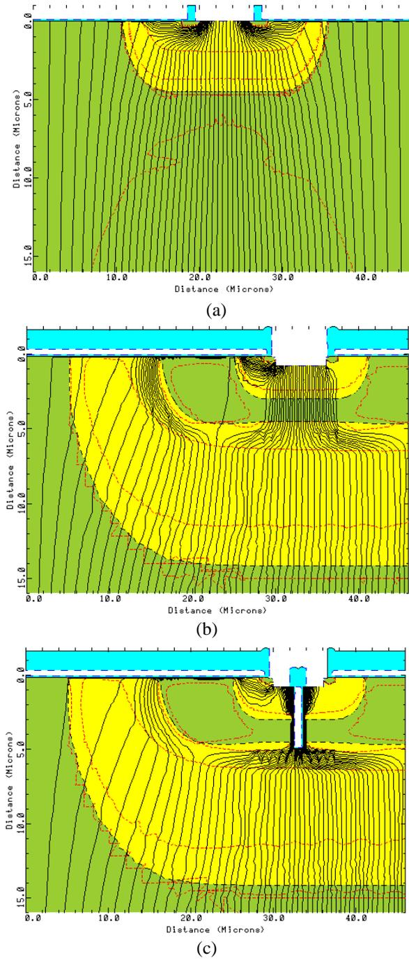
**Fig. 4** Current flow lines of (a) IGBT, (b) CIGBT, and (c) PMOS trench gate CIGBT structure at time=200ns.
