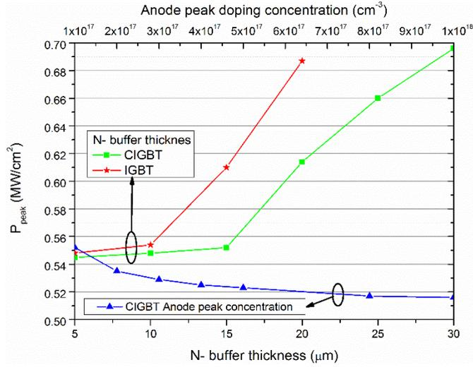
**Fig. 9** Peak power density during turn-off.
