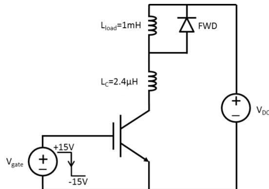
**Fig. 2** Circuit setup of inductive load turn-off simulation.
