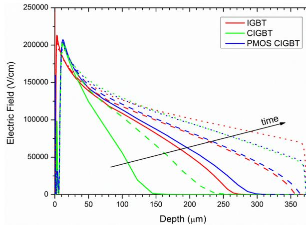
**Fig. 5** Simulated electric fields distribution of structures after gate turn-off (solid line: time=200ns, dash line: time=400ns, and dotted line: time at maximum anode voltage).
