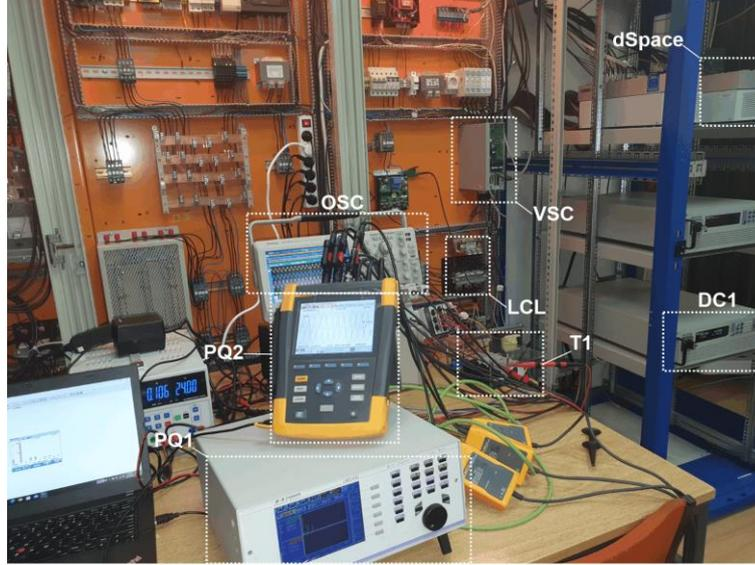
**Fig. 11** Photo of the laboratory microgrid with the main components used in the experiments: VSC – grid inverter, LCL – grid filter interface, DC1 – programmable DC supply, T1 – isolation transformer, PQ1 – power analyser LMG450, PQ2 – Fluke 435 Series II power analyser, OSC – Tektronix digital scope, dSpace - DS 1103 control board
