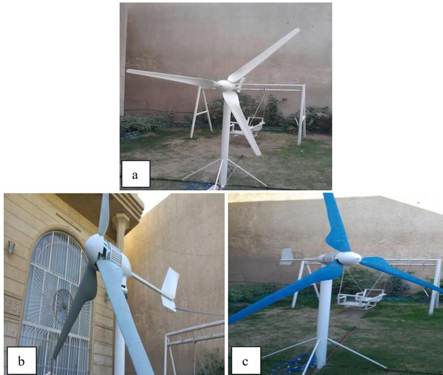
**Fig. 6** Wind turbines (a) with NACA4412 cross-section blades (b) with NACA0012 cross-section blades (c) with EPPLER 317 cross-section blades
