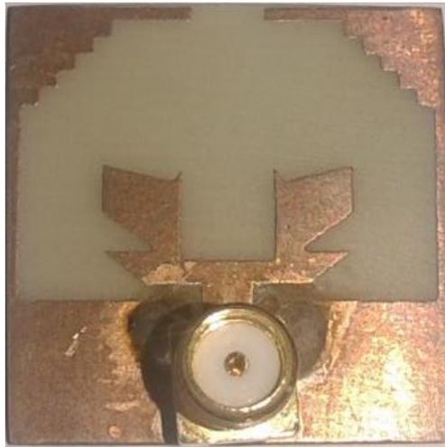
**Fig. 7** Fabricated antenna
