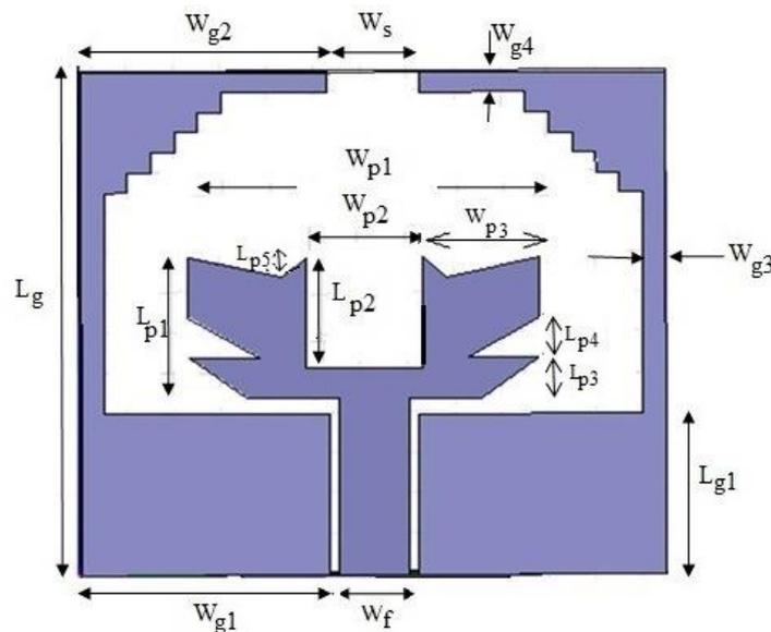
**Fig. 1** Structure of CPW fed slotted antenna
