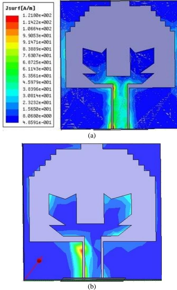
**Fig. 5** Simulated Current density distribution curve (a) 2.8 GHz and (b) 5.9 GHz
