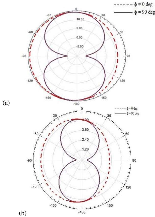
**Fig. 11** The radiation pattern of the designed antenna at (a) 3.3 GHz and (b) 5.82 GHz
