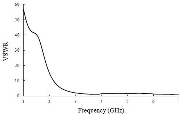
**Fig. 4** Simulated VSWR versus frequency curve
