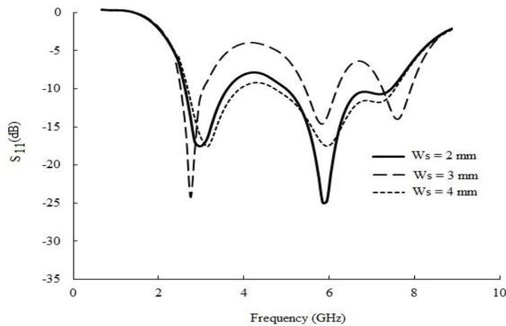
**Fig. 2** Variation of return loss with a ground plane width
