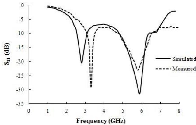
**Fig. 9** Simulated and Measured return loss curve
