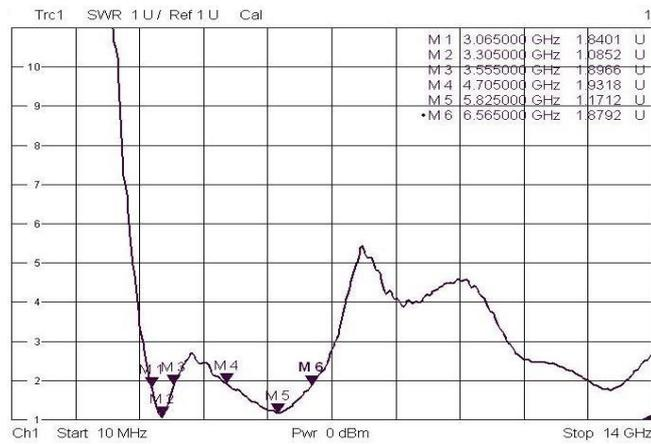
**Fig. 10** Measured VSWR curve
