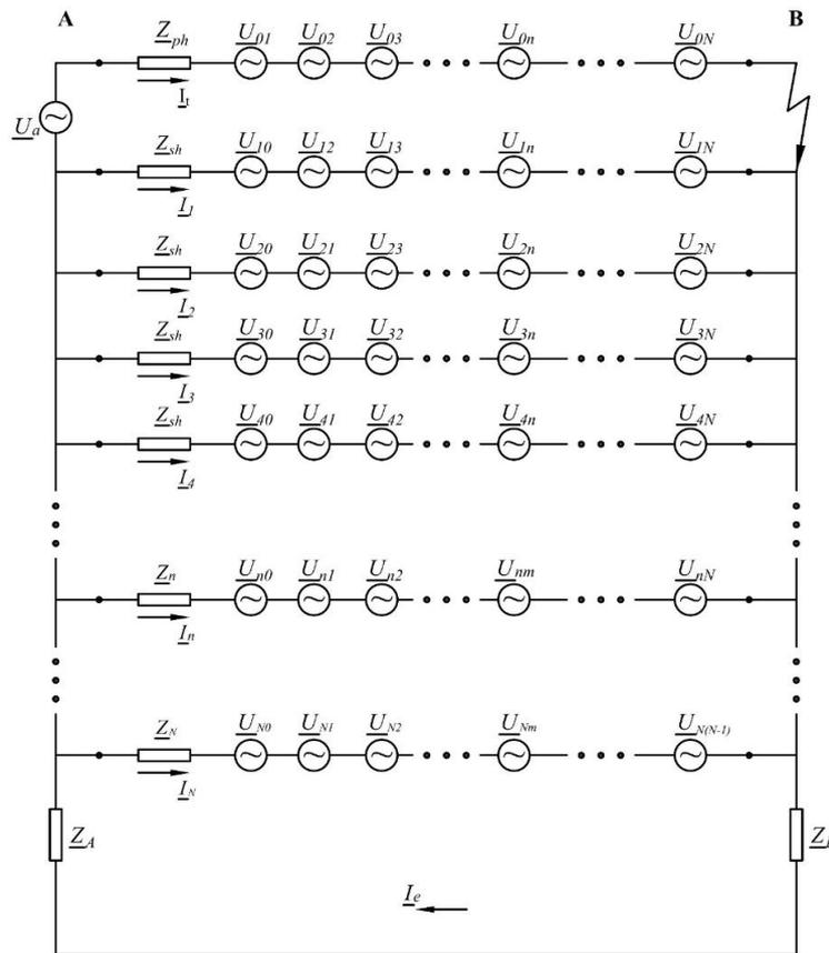
**Fig. 3** Complete equivalent circuit of the assumed HV cable line
