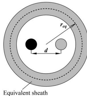
**Fig. 6** Cross-section of the introduced simplified line model
