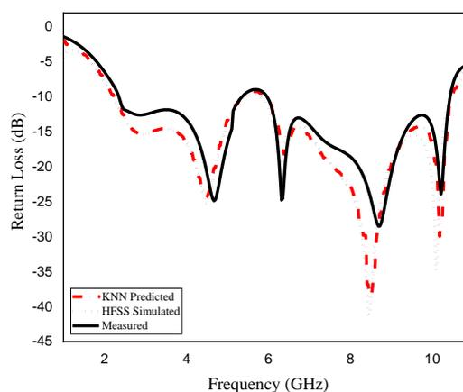
**Fig. 8** Fabricated Antenna **Fig. 9** Return Loss comparison of predicted values from KNN, simulated values from HFSS, and the fabricated prototype
