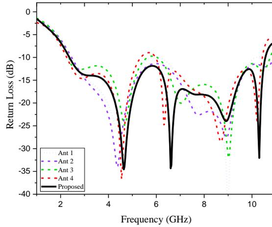
**Fig. 4** Comparison of Return Loss for Ant 1, Ant 2, Ant 3, Ant 4 & Ant 5 (Proposed antenna)
