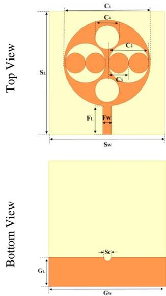
**Fig. 3** Geometry of Ant 5 (Proposed Antenna)
