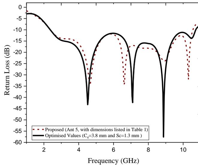
**Fig. 8** Comparison of return loss for proposed design using conventional approach and optimized design using ML
