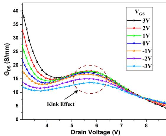
**Fig. 3.** Illustration of abrupt increase in output conductance ( $g_{ds}$ ) as an outcome of kink and traps effect.
