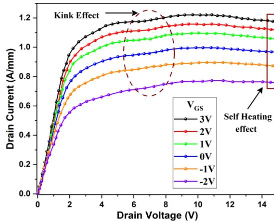
**Fig. 2** The kink effect in an III-Nitride/ $\beta$ -Ga<sub>2</sub>O<sub>3</sub> HEMT at room temperature, where  $V_{GS}$  varies with a step of 1 V from -2 V to 3 V.
