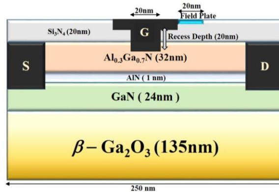
**Fig. 1** Structure and epitaxy details of investigated III-Nitride HEMT on  $\beta$ -Ga<sub>2</sub>O<sub>3</sub> substrate.
