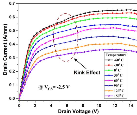
**Fig. 6.** Kink effect in drain characteristics of the HEMT at different temperature values of @  $V_{GS} = -2.5$  V.
