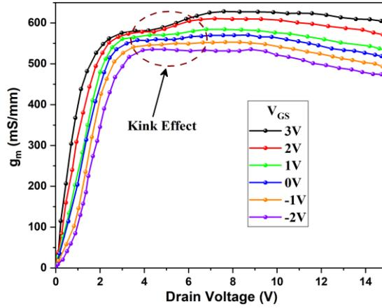
**Fig. 4.** The transconductance ( $g_m$ ) emerged to be compressed as an outcome of kink and traps.
