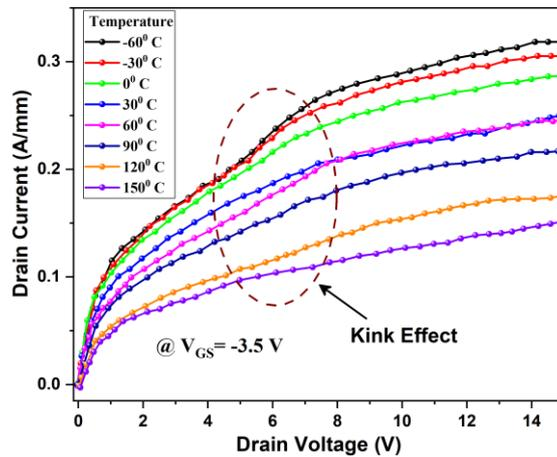
**Fig. 5** Kink effect in drain characteristics of the HEMT at different temperature values of @  $V_{GS} = -3.5V$ .
