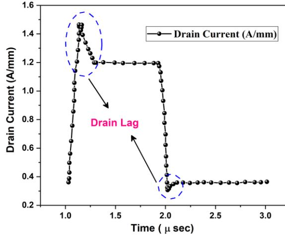
**Fig. 7.** Illustration of Drain Lag in output characteristics of the HEMT at different temperature values.
