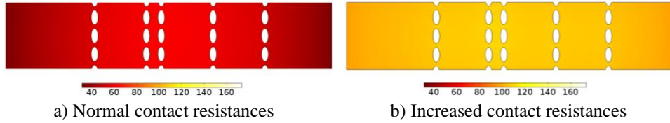
Fig. 12 Distribution of the thermal field (°C) in fuse link at time t=10\text{ min} and rated current of I_n=50\text{ A}
