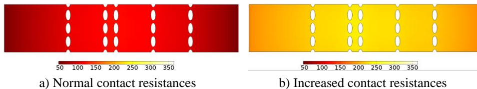
Fig. 20 Distribution of the thermal field (°C) in the fuse link at time t=1 \text{ min} and test current of I=75 \text{ A}
