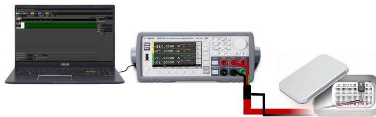
Fig. 3 Schematic representation of the I - V measurement setup
