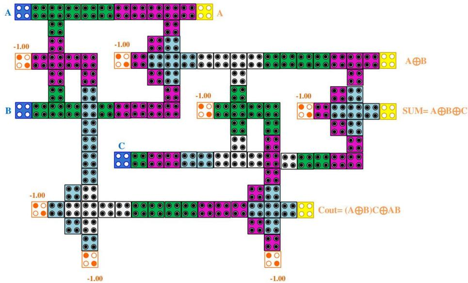
**Fig. 10** Layout of the RFA circuit in [28]
