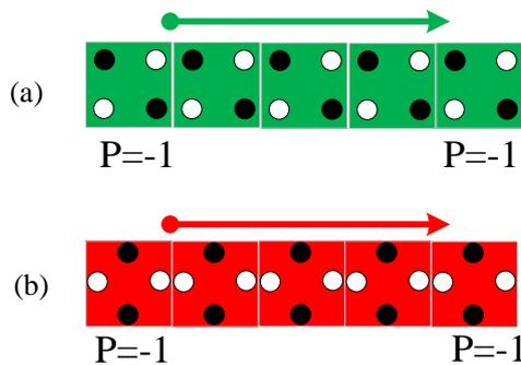
**Fig. 2** Wires in the QCA technology a) normal, b) with 450 rotations
