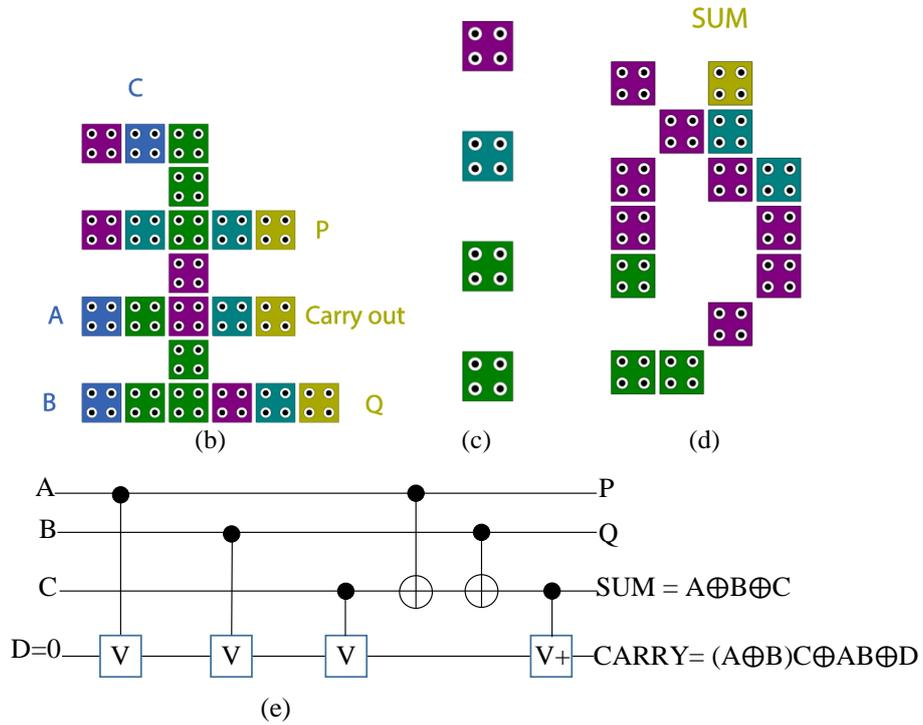
**Fig. 14** Suggested RFA a) 3 layers, b) 1st layer, c) 2nd layer, d) 3rd layer e) quantum circuit
