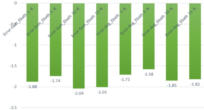
**Fig. 18** Error of sum and average energy of our RFA circuit for different temperatures
