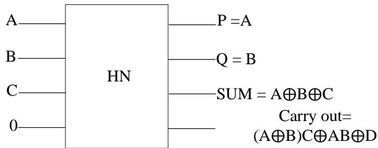
**Fig. 13** Block diagram of the proposed RFA using HN gate
