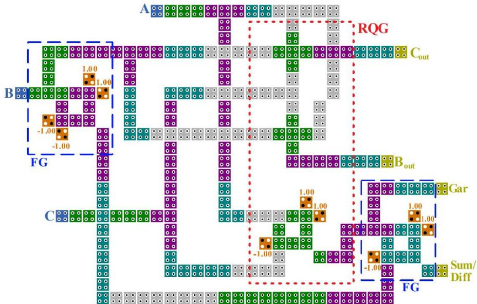
**Fig. 9** Layout of the RFA circuit in [27]
