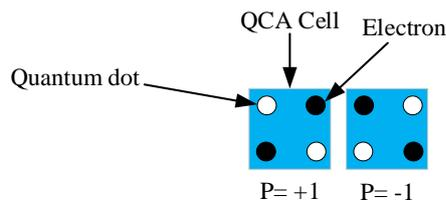
**Fig. 1** The QCA cell structure and its stable stats
