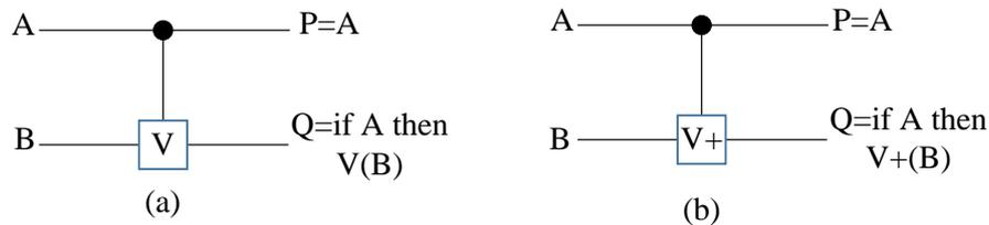
**Fig. 7** Controlled gates a) V gate, b) V+ gate
