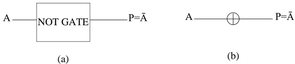
**Fig. 5** Reversible NOT gate a) logic diagram, b) quantum circuit
