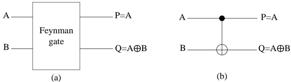
**Fig. 6** Feynman gate a) logic diagram, b) quantum circuit
