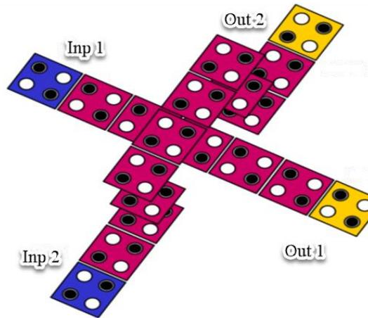
**Fig. 3** QCA multilayer crossing wire
