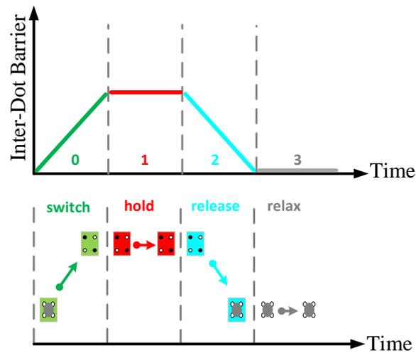
**Fig. 4** QCA clocking with four phases
