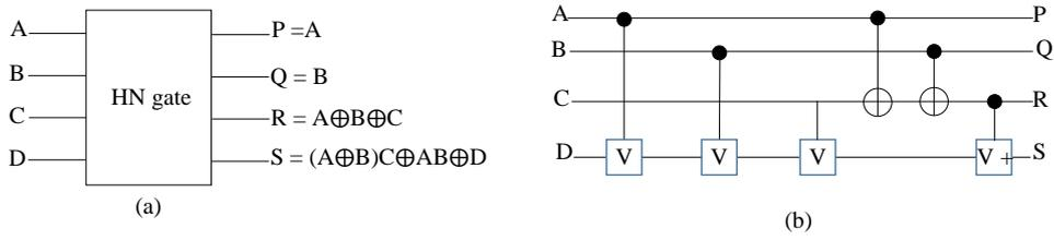
**Fig. 8** HN gate a) logic diagram b) quantum circuit
