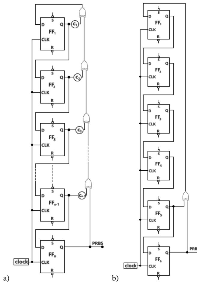
Fig. 1 Generator of direct PRBS for a) an arbitrary resolution  $n$ ; b) resolution  $n = 6$
