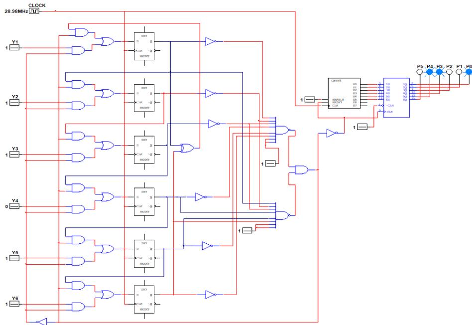
**Fig. 6** Simulation of the serial pseudorandom/natural code converter in NI Multisim software for resolution  $n = 6$
