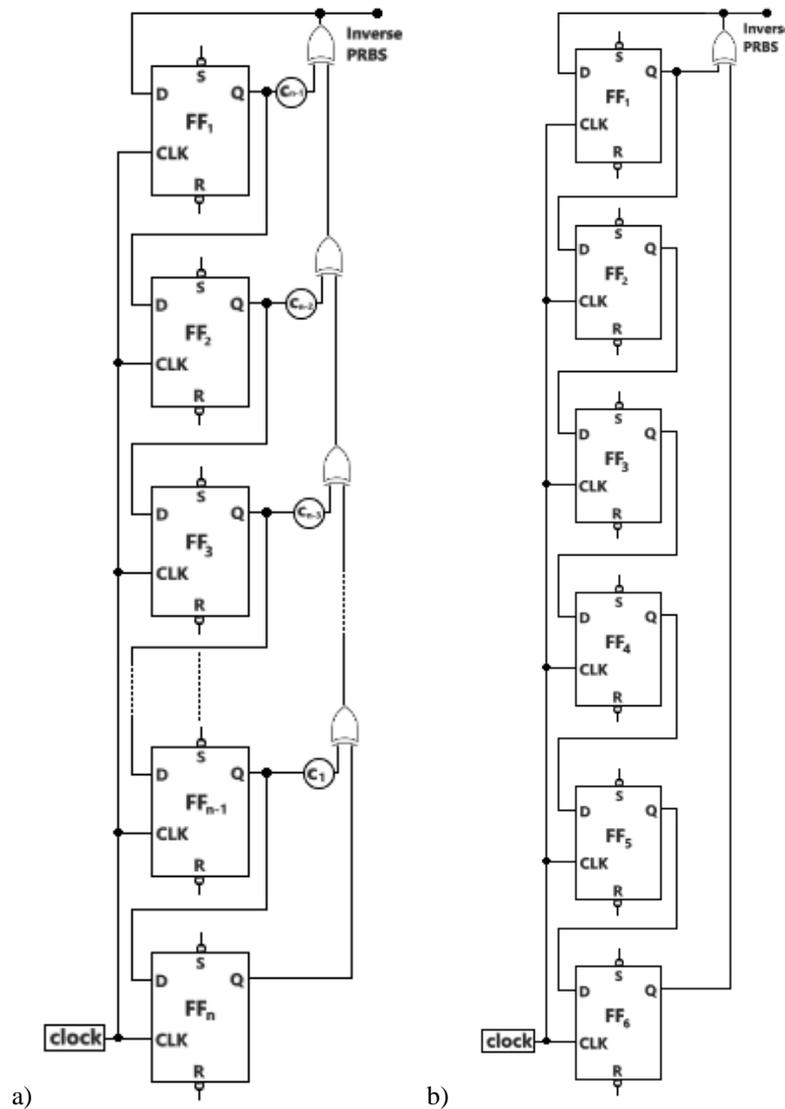
**Fig. 2** Generator of inverse PRBS for a) an arbitrary resolution  $n$ ; b) resolution  $n = 6$
