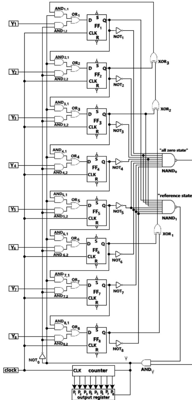
Fig. 5 The block diagram of the serial pseudorandom/natural code converter for resolution  $n = 8$
