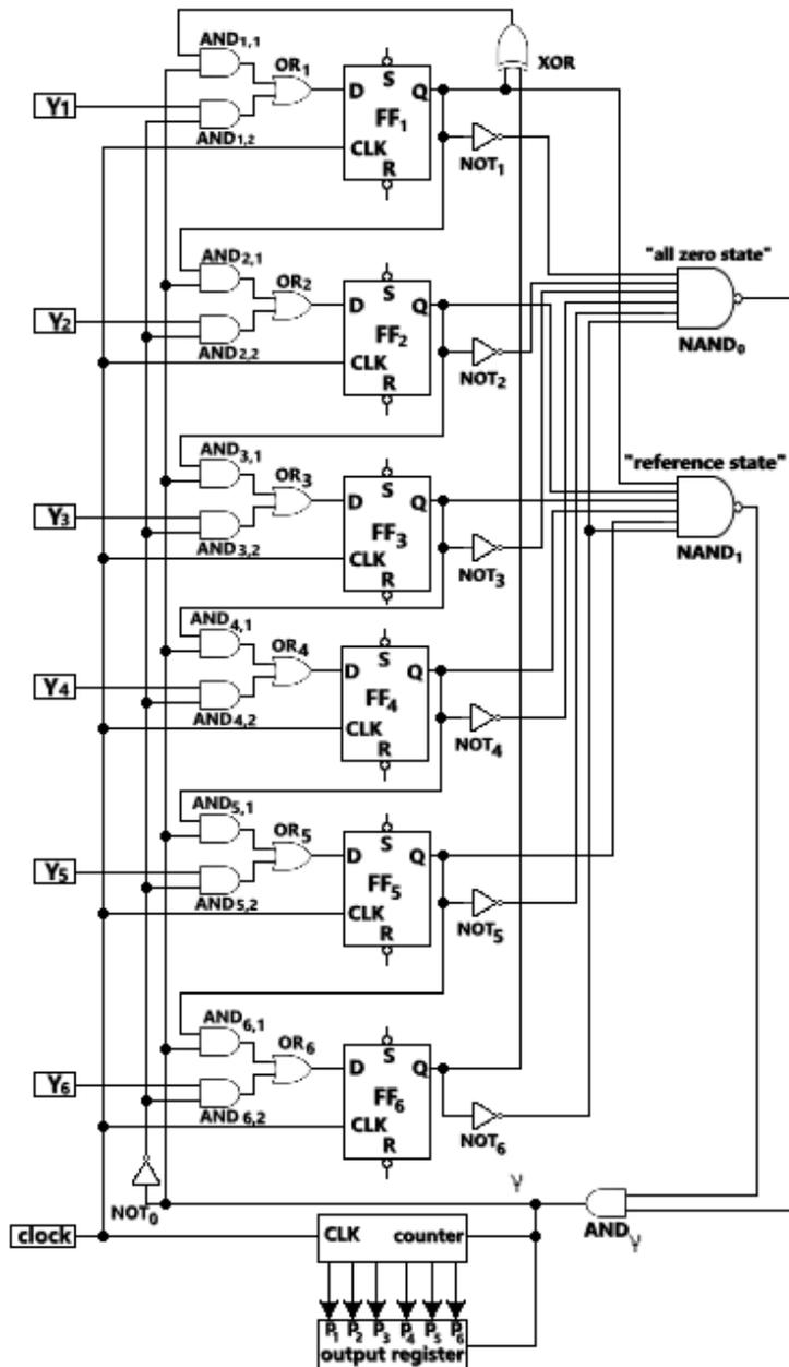
Fig. 4 The block diagram of the serial pseudorandom/natural code converter for resolution  $n = 6$
