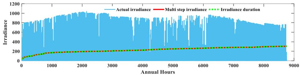
Fig. 3 Multistep solar irradiance curve
