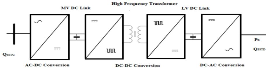
Fig. 5 Schematic arrangement of Solid State Transformer [35]
