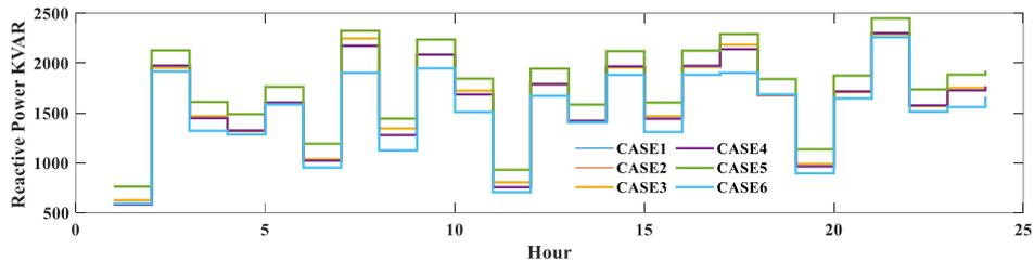
**Fig. 11** Reactive power decrement after SST and DG placement of all the test cases
