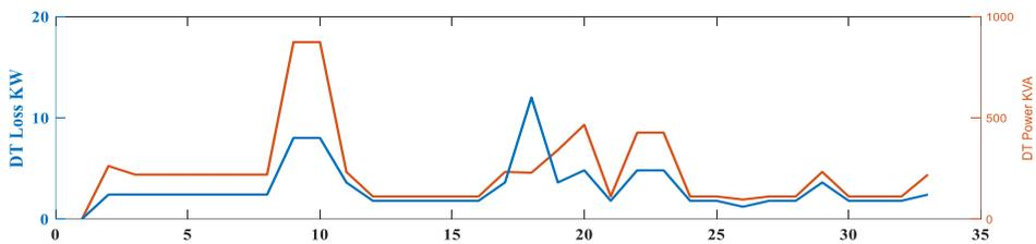
Fig. 8 DT losses along with installed capacity
