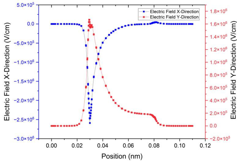
**Fig. 4** Graph illustrating the spatial variation of Electric Field components (X and Y directions) within a TFET. X-Direction field shows a sharp peak ( $\sim 1.8 \times 10^6$  V/cm), indicative of the tunneling junction. Y-Direction field exhibits a smaller magnitude and likely influences lateral carrier transport.
