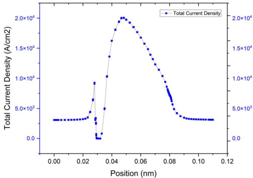
**Fig. 11** Total Current Density diagram for the simulated TFET device
