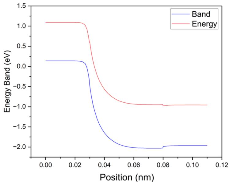
**Fig. 7** Energy Band Diagram for the simulated TFET device. The band bending shows a significant potential drop ( $\sim 1.5$  eV) across the tunneling junction, enabling band-to-band tunneling.
