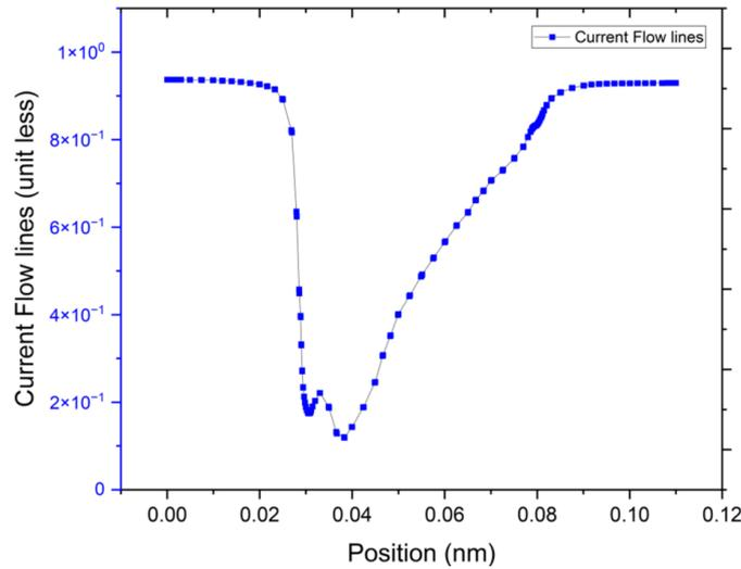
**Fig. 2** Graph illustrating the variation of Current Flow Lines within a simulated Tunnel Field Effect Transistor (TFET) device. The peak in current flow lines occurs as of the active tunneling region where electrons quantum-mechanically tunnel through the bandgap.
