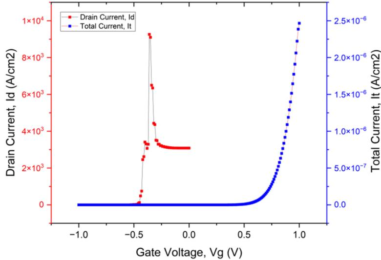
**Fig. 8** Current Vs Voltage diagram for the simulated TFET device. Drain Current ( $I_D$ ) exhibits a steep subthreshold slope ( $\sim 60\text{mV/dec}$ ) and a peak current density of  $1 \times 10^4 \text{ A/cm}^2$ . Total Current ( $I_t$ ) shows a slight offset due to leakage currents.
