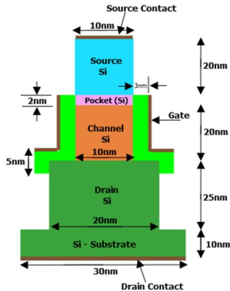
**Fig. 1** Simulated TFET Device Structure
