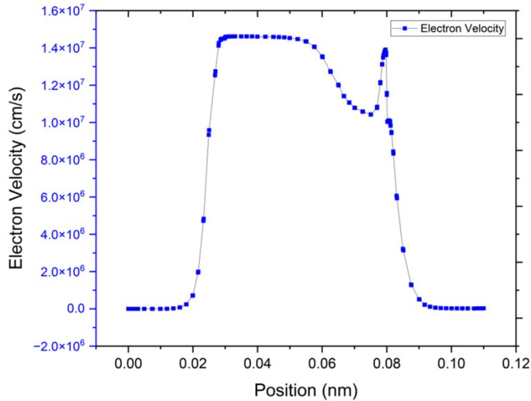
**Fig. 6** Graph illustrating the spatial variation of Electron Velocity within a Tunnel Field Effect Transistor (TFET) device. A sharp peak in electron velocity ( $\sim 1.5 \times 10^7$  cm/s), indicating the tunneling junction, and regions of reduced velocity, potentially attributed to carrier scattering or variations in the electric field.
