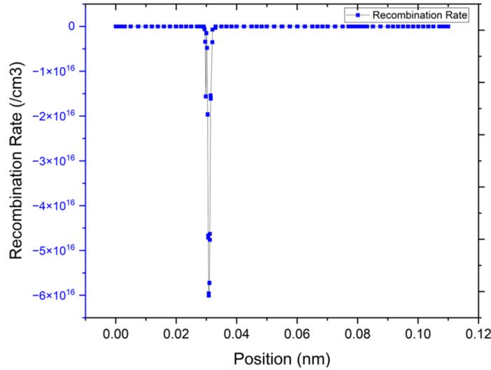
**Fig. 5** Graph illustrating the spatial variation of Recombination Rate within a TFET. A sharp peak in recombination rate ( $\sim -5 \times 10^{16} / \text{cm}^3$ ) is observed, indicating a region of high carrier recombination activity, likely influenced by localized defects or carrier trapping.
