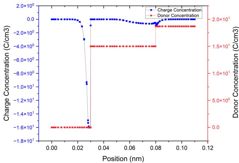
**Fig. 3** Graph illustrating the distribution of Charge Concentration and Donor Concentration for a simulated TFET device. The blue line represents the Charge Concentration, while the red line represents the Donor Concentration. The x-axis represents the position along the device channel, measured in nanometers (nm).
