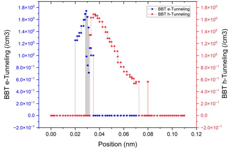
**Fig. 9** Graph illustrating the Band-to-Band Tunneling (BBT) rates for electrons (e-Tunneling) and holes (h-Tunneling) within a TFET. Peak e-Tunneling rate ( $\sim 1.6 \times 10^9 / \text{cm}^3$ ) occurs at  $\sim 0.04$  nm, while h-Tunneling peak is lower and shifted slightly.
