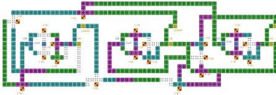
Fig. 12 QCA Designer layout of 3-bit sequential counter
