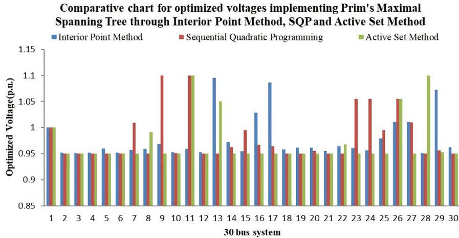
**Fig. 12** Comparative analysis for optimized voltages implementing Prim's Maximal Spanning Tree using the Interior Point Method, SQP and Active Set Method.
