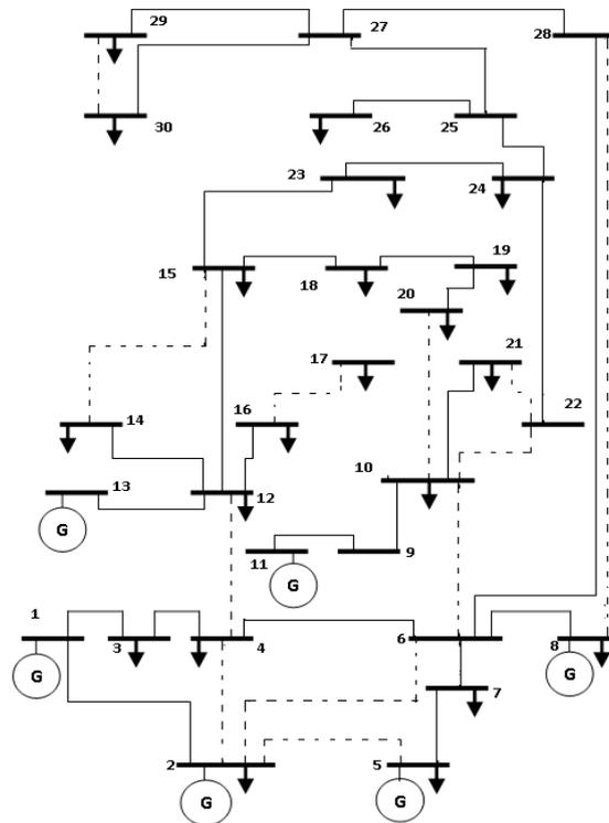
**Fig. 5** Optimal configuration of Prim's Maximal Spanning Tree through implementing Interior Point Method
