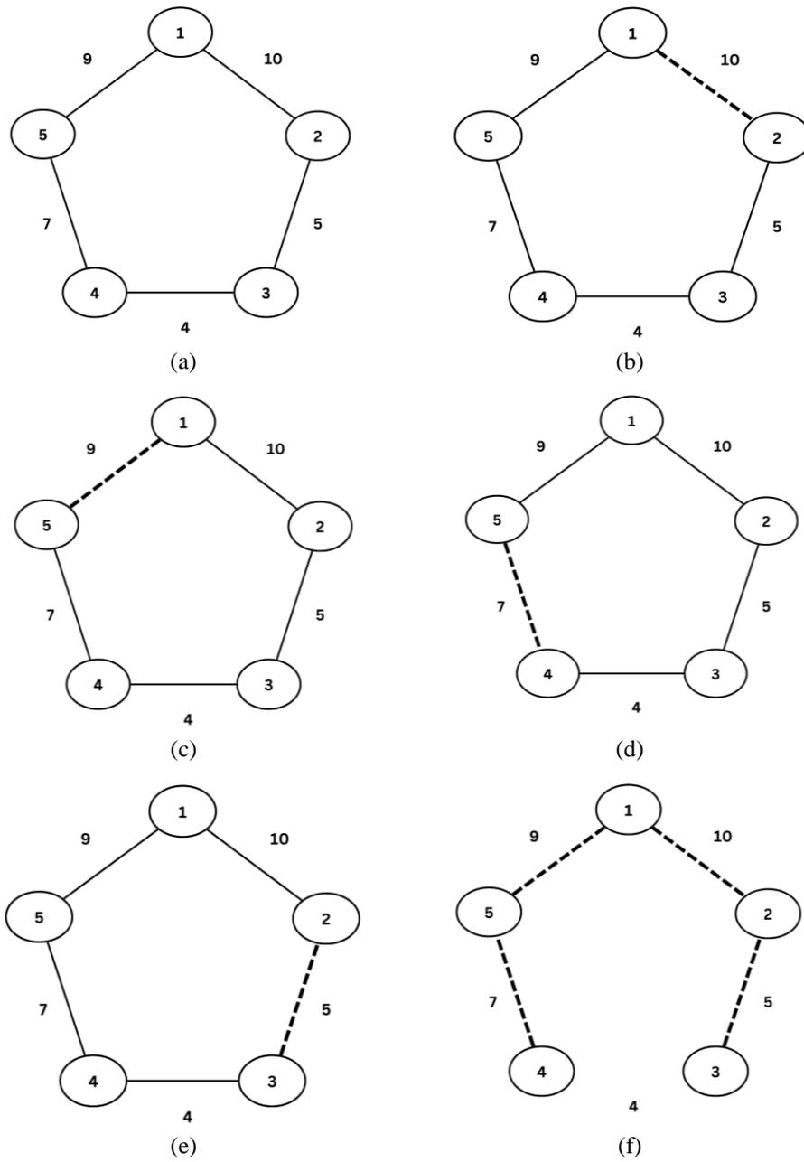
**Fig. 2(a-f)** Network reconfiguration using Prim’s Maximal Spanning Tree
