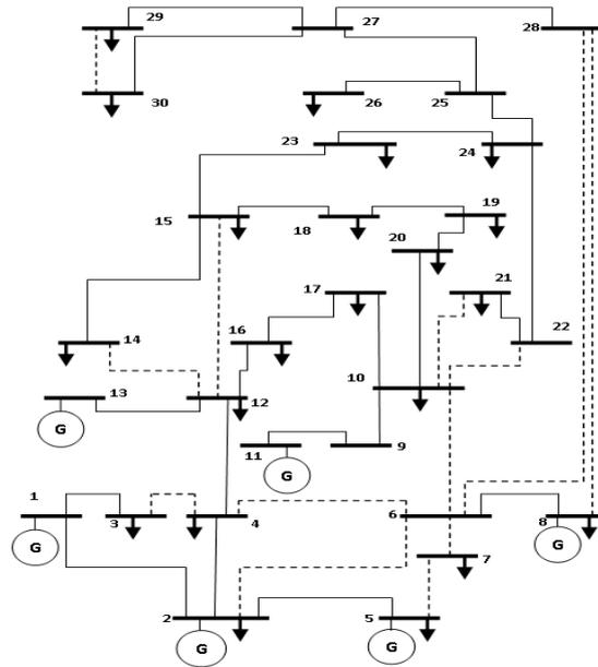
**Fig. 9** Optimal configuration of Prim's Maximal Spanning Tree through the implementation of Active Set
