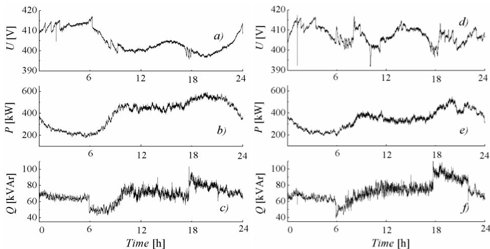
**Fig. 2** Voltage a), real b) and reactive power c) curves during Sunday, and voltage d), real e) and reactive power f) curves recorded on Friday
