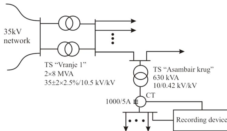
**Fig. 1** Principal diagram of device connections in considered TS
