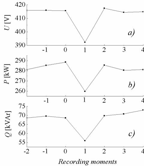
**Fig. 3** Two subsequent voltage changes a), and real b) and reactive c) power responses
