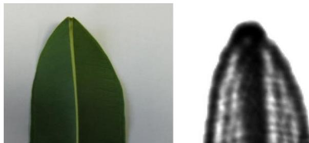
**Fig. 6** Visual and THz image in transmission mode
