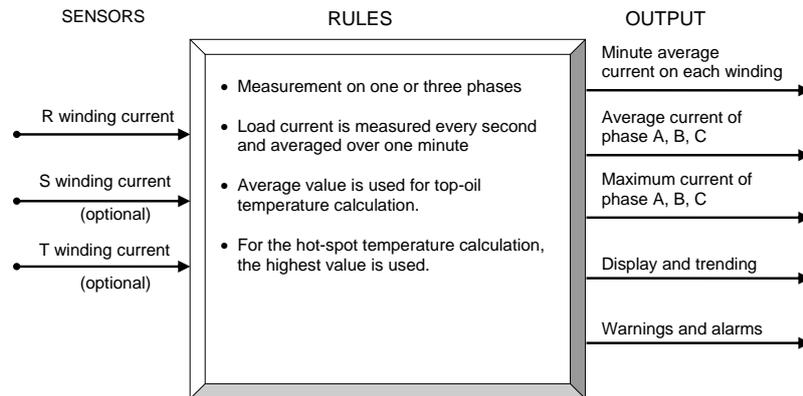
**Fig. 1** Load current model
