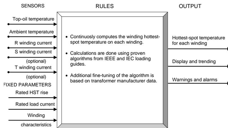
**Fig. 2** Winding temperature model
