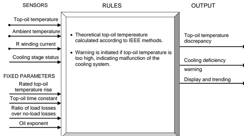
**Fig. 4** Cooling efficiency model
