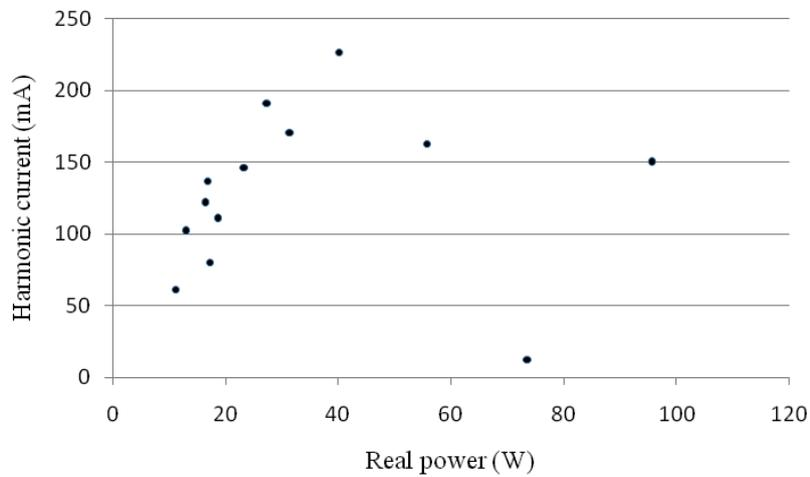
**Fig. 2** Load distribution of the tested appliances in P-I<sub>H</sub> plane
