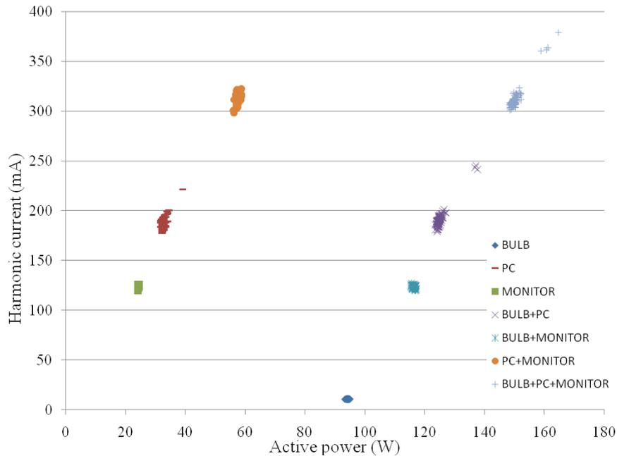
**Fig. 3** Distribution of bulb, monitor and PC in the P- $I_H$  feature space
