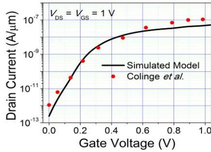
**Fig. 2** Comparison of  $I_{D,LIN}$  with respect to  $V_{GS}$  plot for SG-OI JLCT at  $V_{DS} = 1$  V and [13] with simulation  $L_G = 20$ -nm,  $\phi_M = 5.1$  eV,  $N_D = 1.5 \times 10^{19} \text{ cm}^{-3}$
