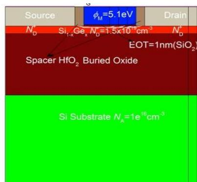
**Fig. 1** Cross sectional view of SG-OI JLCT
