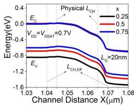
**Fig. 4** Energy with respect to Distance “X” along the channel for SG-OI JLCT is shown. For  $\text{Si}_{1-x}\text{Ge}_x$  channel ( $x = 0.25, 0.5, 0.75$ ),  $V_{\text{DSAT}} = 0.7$  V and  $T_{\text{Si}} = 5$  nm is given.
