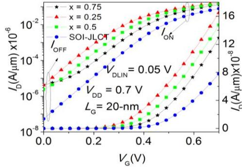
Fig. 3 Comparative Analysis of  $I_{D,LIN}$  with respect to  $V_{GS}$  is shown for SOI JLCT and SG-OI JLCT. With  $\phi_M = 5.1$  eV,  $N_D = 1.5e19$  cm<sup>-3</sup> and  $L_G = 20$ -nm
