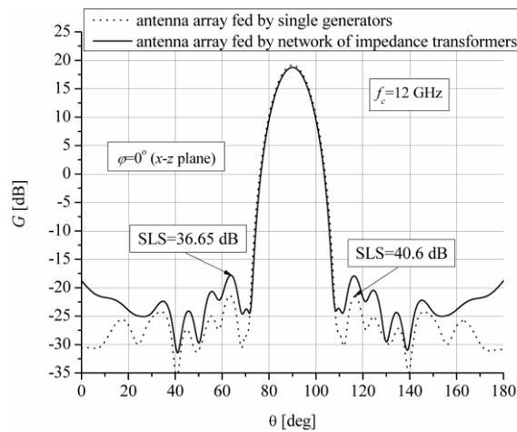
**Fig. 3** Radiation pattern of printed antenna array in corner reflector with angle of  $90^\circ$  in E plane
