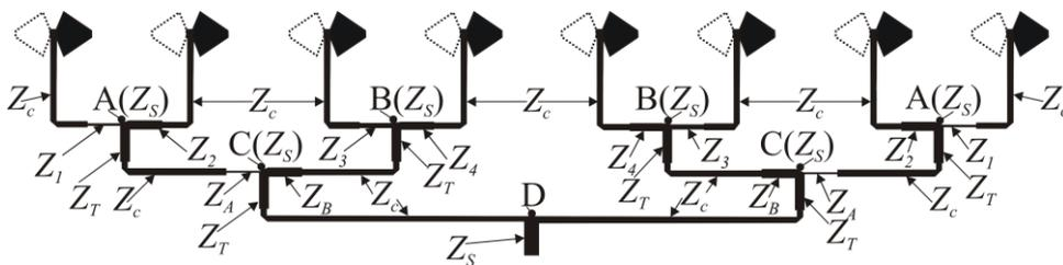
**Fig. 2** Feeding network of impedance transformers for antenna array with high side lobe suppression
