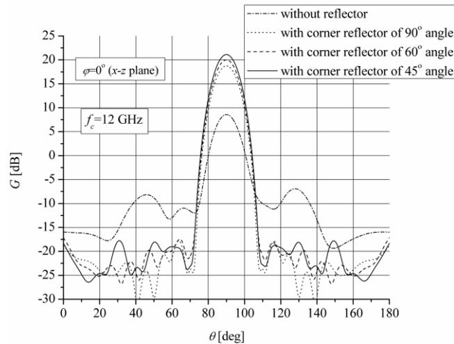
**Fig. 11** Simulated radiation pattern in E plane of antenna arrays without reflector and with corner reflector with different angles
