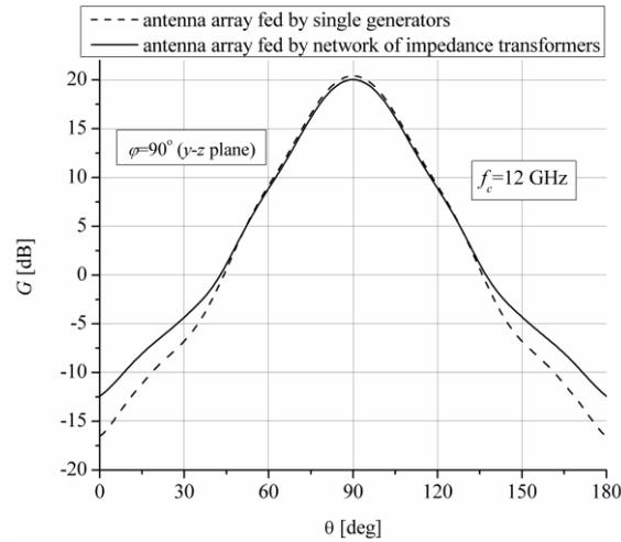
**Fig. 6** Radiation pattern of printed antenna array in corner reflector with angle of  $60^\circ$  in H plane
