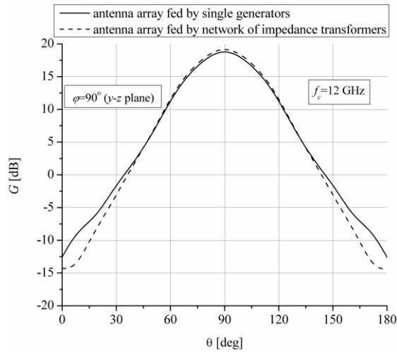
**Fig. 4** Radiation pattern of printed antenna array in corner reflector with angle of  $90^\circ$  in H plane
