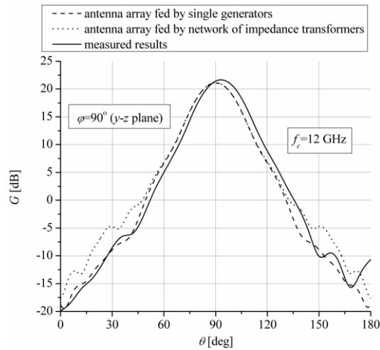
**Fig. 8** Radiation pattern of printed antenna array in corner reflector with angle of  $45^\circ$  in H plane
