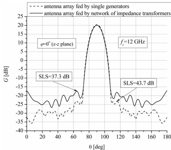
**Fig. 5** Radiation pattern of printed antenna array in corner reflector with angle of  $60^\circ$  in E plane
