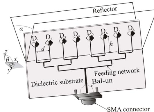
**Fig. 1** Printed antenna array of eight symmetrical pentagonal dipoles with feeding network, balun and reflector
