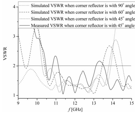
**Fig. 10** VSWR of antenna arrays in corner reflector with different angles
