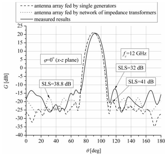
**Fig. 7** Radiation pattern of printed antenna array in corner reflector with angle of  $45^\circ$  in E plane
