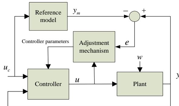
**Fig. 1** Block diagram of model reference adaptive control
