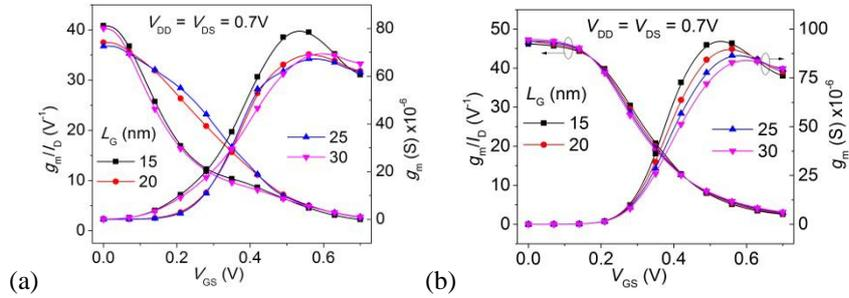
**Fig. 3**  $TGF$  and  $g_m$  as a function  $V_{GS}$  (a) JL FinFET and (b) Wavy-JL FinFET for different  $L_G = 15$ -30 nm at  $N_D = 1.7 \times 10^{19} \text{ cm}^{-3}$ ,  $\phi_M = 4.6 \text{ eV}$  and  $x = 0.25$ .
