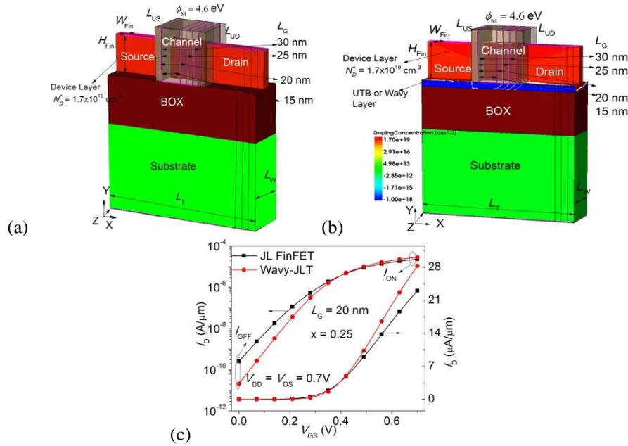
**Fig. 1** A 3D representation of (a) Conventional JL FinFET, (b) Wavy-JL FinFET at  $L_G = 15\text{-}30 \text{ nm}$  (c)  $I_D$ - $V_{GS}$  characteristics of Conventional and Wavy JL FinFET at  $L_G = 20 \text{ nm}$  and  $x = 0.25$ .
