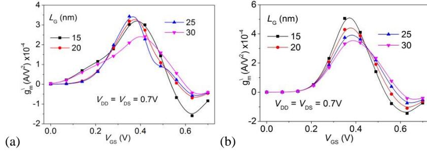
**Fig. 4**  $g_m^{\parallel}$  as a function  $V_{GS}$  (a) JL FinFET and (b) Wavy-JL FinFET for different  $L_G = 15-30$  nm at  $N_D = 1.7 \times 10^{19}$  cm $^{-3}$ ,  $\phi_M = 4.6$  eV and  $x = 0.25$ .
