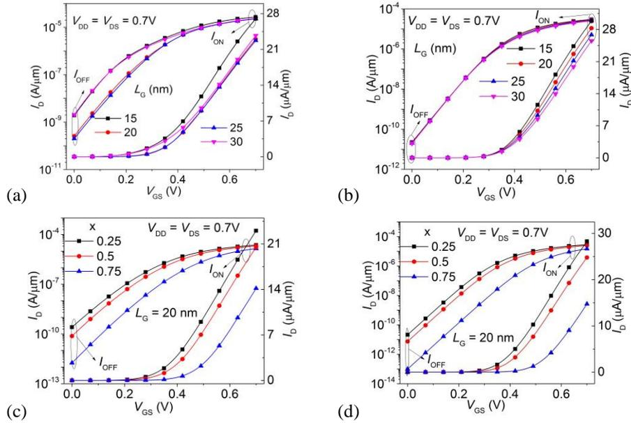
**Fig. 2** Transfer characteristics of (a) JL FinFET and (b) Wavy-JL FinFET for varying  $L_G = 15$ -30 nm at  $N_D = 1.7 \times 10^{19} \text{ cm}^{-3}$ ,  $\phi_M = 4.6 \text{ eV}$ .
