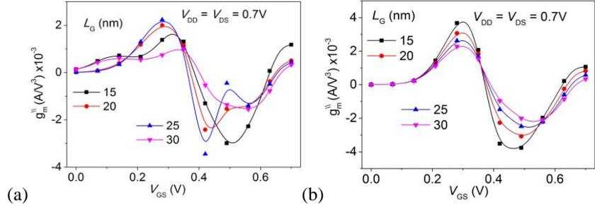
**Fig. 5**  $g_m^{\parallel}$  as a function  $V_{GS}$  (a) JL FinFET and (b) Wavy-JL FinFET for different  $L_G = 15-30$  nm at  $N_D = 1.7 \times 10^{19}$  cm $^{-3}$ ,  $\phi_M = 4.6$  eV and  $x = 0.25$ .
